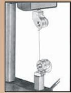
Spool Grip for Fibres, Filaments, Wires, etc.
