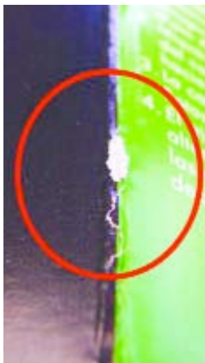
Fig. 3 On the typical corrugated container, it’s the inner liner that usually cracks. When running jobs that consist of litho laminated labels mounted to combined board the crack tends to occur on the printed outside liner.
