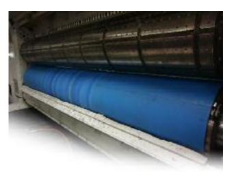
REPAIRING DIES WITH UNLIKE RULE HEIGHTS AND PROFILES WILL CAUSE PREMATURE ANVIL WEAR.
